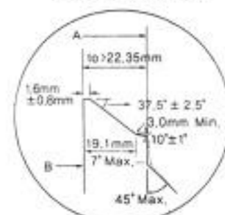
BEVEL FOR WALL THICKNESS(to) GREATER THAN 0.68 IN.(22.35mm)
