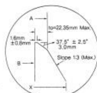
BEVEL FOR WALL THICKNESS(to) 0.68" IN.(22.35mm) OR LESS.
